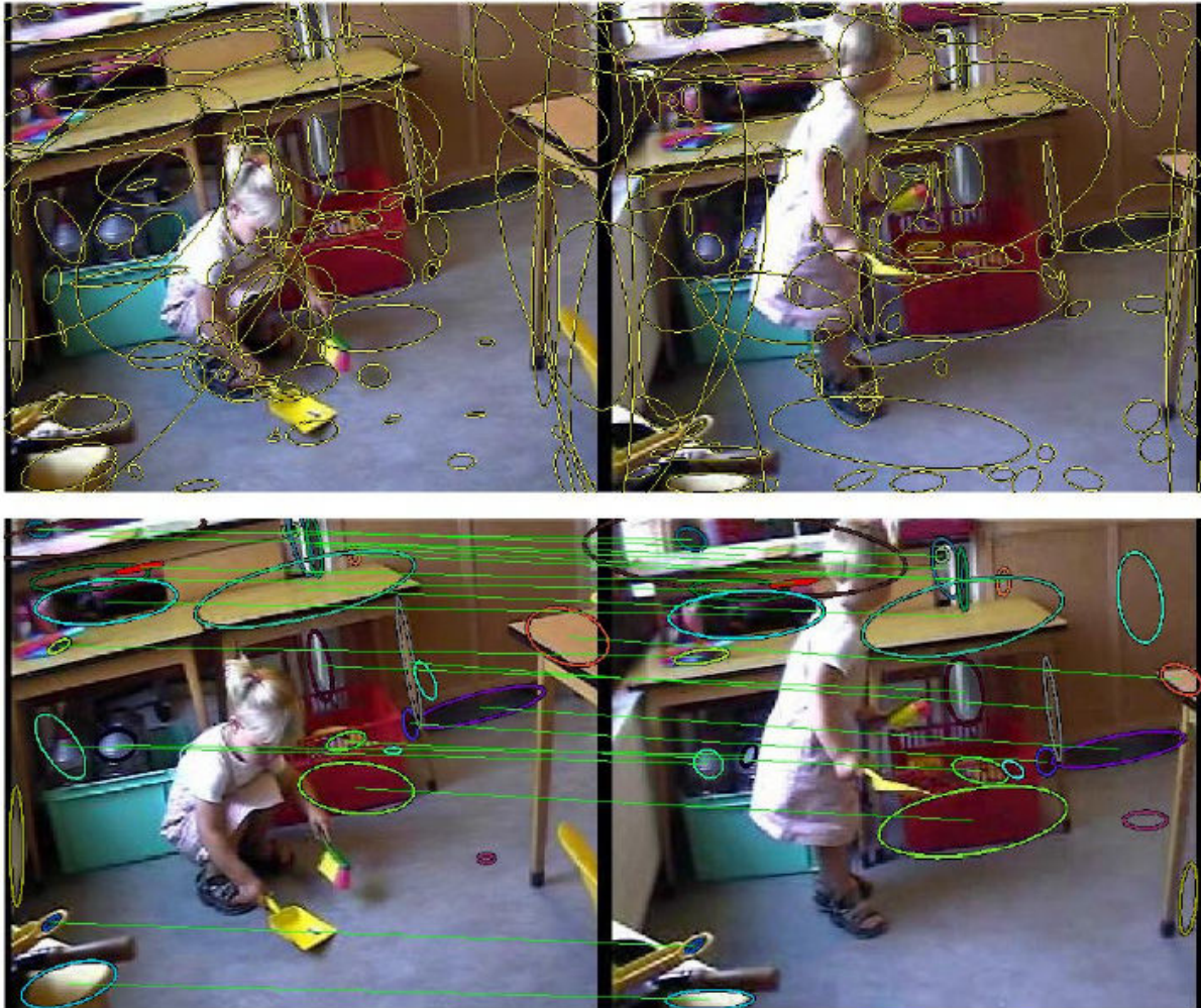
Figure 5: MSSR region detection. On top all detected regions, in the bottom corresponding regions and spatially consist matches.
