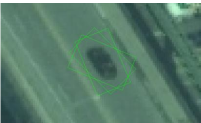
Figure 2. Example of a vehicle that is detected in 3 different rotations. Only the detection with the highest confidence is maintained (the one in the middle).
