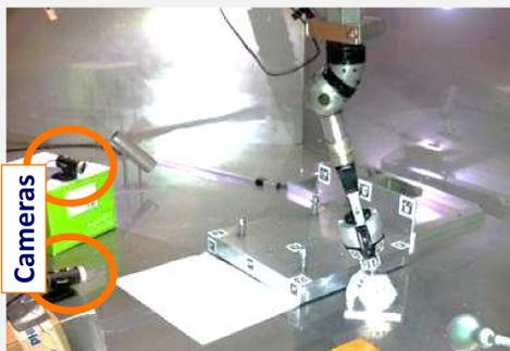
Slave manipulator holds bolt runner. Front and side view cameras observe the scene. A single camera shows a frontal close-up view of the test setup on the workbench.
