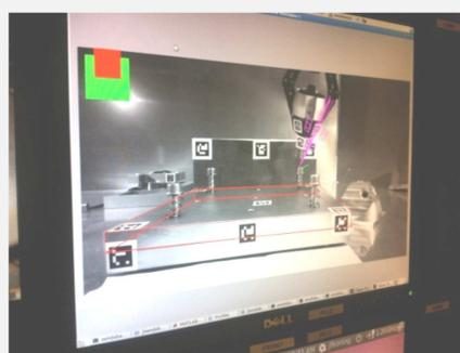
Operator view of the 4-bolt benchmark shows artificial depth cue: the red bar on the top left, and artificial task cue: a green line and magenta circle indicating the target location at the bolt head.
